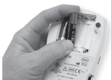
Insert 4 AAA batteries according to the diagram inside the battery compartment.
