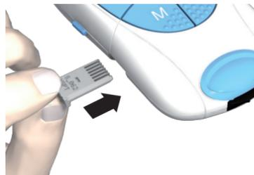
Make sure the meter is off. With the code number facing up, insert the code chip into the code chip slot until it snaps into place.
