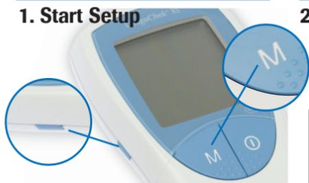
To set the date and time, use these buttons: **M** to change a setting and **⏏** (SET) to accept a setting.
