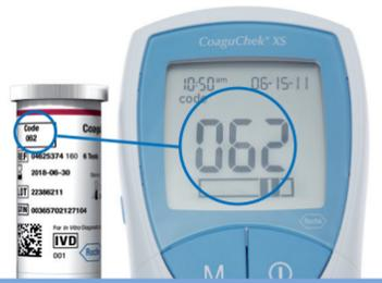
Confirm that the number displayed matches the number on the test strip container, then press **M**.
